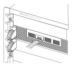
Figure 23: Installed CFP2 Module (BlackDiamond X8 series switch)
